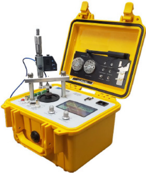
Figure 5. Proximity probe kit installed on AT2040
