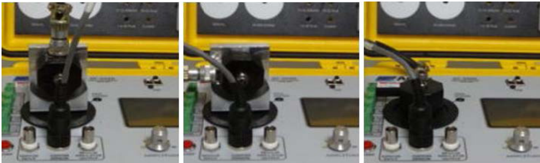
Figure 42. Sensor positioning and connection method
