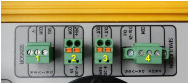
Figure 82. 4-20mA ("3") and proximity probe simulator connectors ("4")
